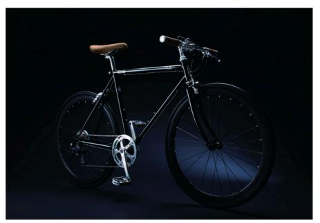
The Tern Roji bikes are practical and designed for daily riding, with simple 1 x 8 gearing and braze-ons for fenders and racks. But they also include a number of design details such as beautiful lugged forks, fin-shaped tubes, Dura-Ace down-tube shifters, and
