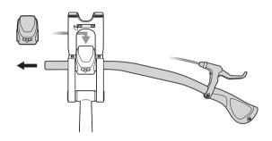
4. Tighten the Stem and install the Grip, Brake Lever, and Gear Shifter, tightening all to manufacturer specifications.
