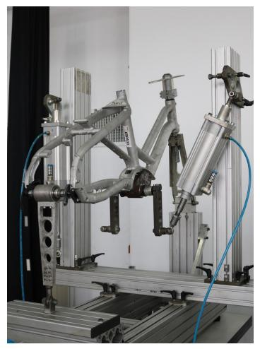
The GSD and the HSD have both passed the EFBE Tri-Test up to the claimed load limits of 200 kg and 170 kg respectively, which means they meet and exceed the German cargo bike standard.
