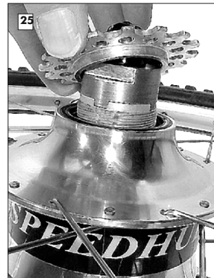
Replace the new/rotated sprocket (with undamaged seal surfaces) as shown in the Owners Manual.
