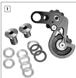
The Rohloff DH chain tensioner comes with 2 mounting bolts and 9 distancing washers (4 x 1mm, 2 x 3mm, 3 x 0.2mm).
