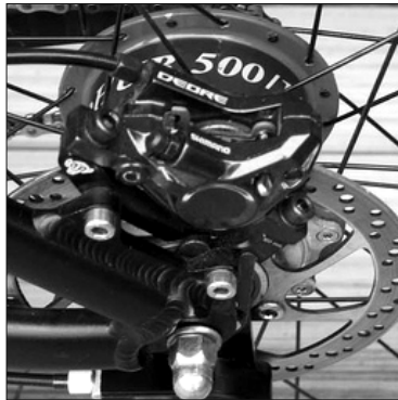
Rohloff SPEEDHUB 500/14 TS DB OEM2 mounted with the Rohloff MONKEY BONE (IS-PM Adapter) and a TS 2000 disc brake
