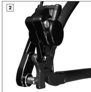
Mounted Rohloff SPEEDBONE, view from inside the frame.
