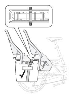
Use the Pannier Adapter to secure the Cargo Hold 37 Panniers straps when using a Thule® Yepp Maxi child seat in the rear window of a GSD.
