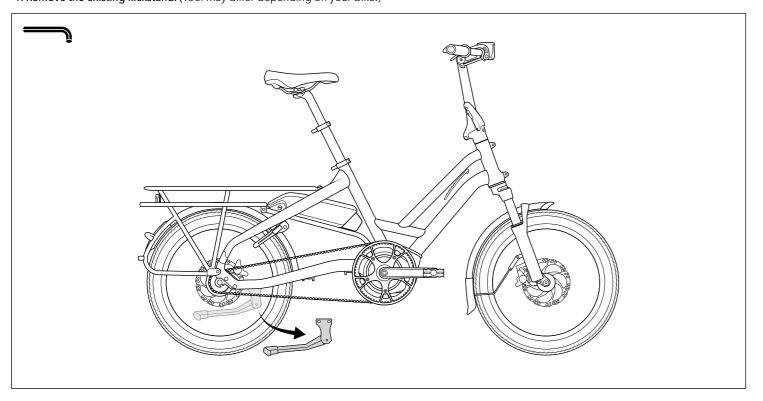
2. Identify the HSD frame by locating the kickstand mount in front of the rear wheel.
