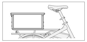
2. Install the Base Plate to the inside of the Soft Crate Mini.
