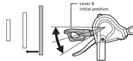
Gears can be shifted by pushing or pulling the lever.
