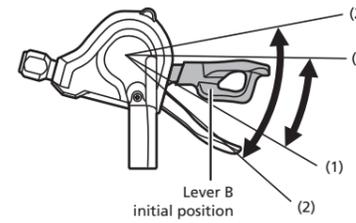
Gears can be shifted by pushing or pulling the lever. Some models have two-step gear shifting.
