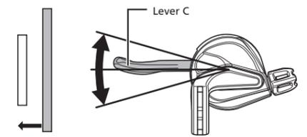
Gears can be shifted by pushing or pulling the lever.
