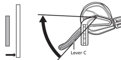
\* After shifting, the lever is kept in position C-2.
