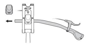
4. Tighten the Stem and install the Grip, Brake Lever, and Gear Shifter, tightening all to manufacturer specifications.
