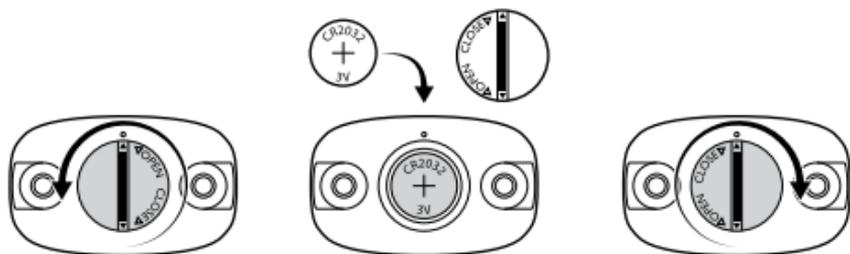
To replace the battery, remove the Battery Cover by turning counter-clockwise using a coin and place the battery inside with the negative terminal facing down (i.e., the front of the battery should be visible through the Battery Cover Hole).
