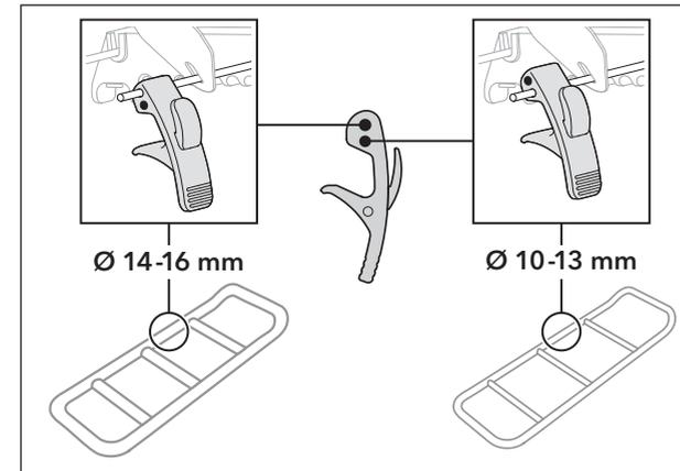
2. Insert both rods into the appropriate holes and reinsert rods into the bracket.
