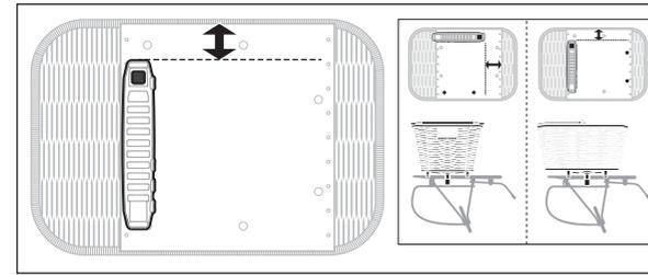
3. Place one bracket in the mounting holes in the desired mounting orientation.
