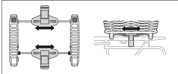
2. Set the basket down and check if the levers can close. If not, change the position of the levers anywhere along the spring rod and test again.
