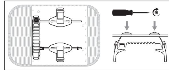
4. Reinsert the rods into the bracket.
