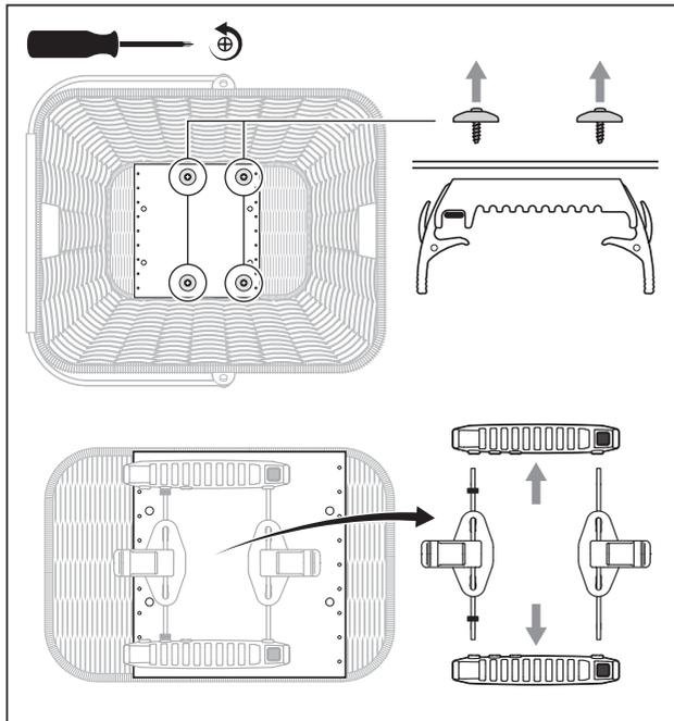
1. Loosen screws of brackets with Cross-Head Screwdriver.
