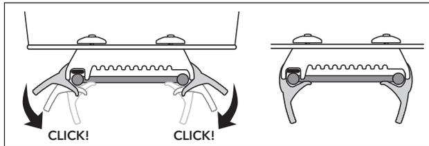
3. Close the levers and make sure the levers click inwards. Please note that the rack tube may sit at different locations on the TopKlip on the non-red side of the basket.
