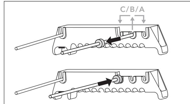
The Market Basket can fit racks between 9 - 16 cm wide. Out of the box, the Market Basket has already been set up to mount on a Tern or BioLogic rack or a rack that is between 11 - 13 cm wide (B). Measure the width of the rack from side to side to determine which setting (A, B or C) to use.
