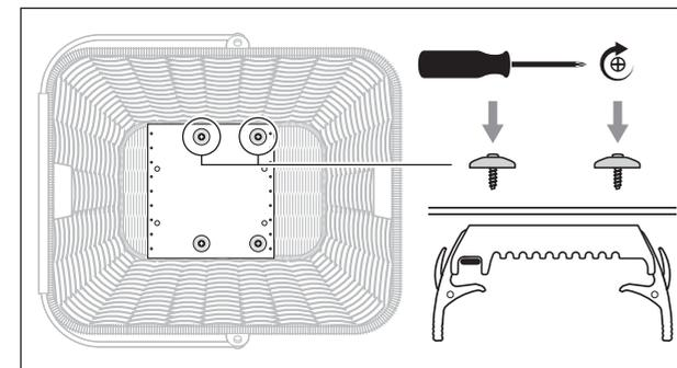
3. Tighten the screws (Max 2 Nm).
