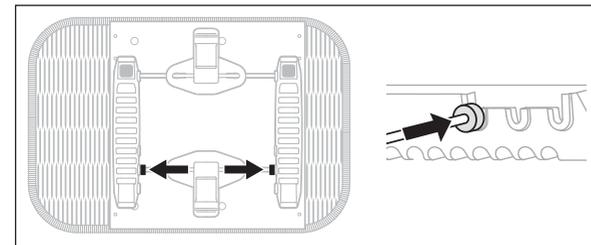
7. Slide the rubber retainer rings against the brackets.
