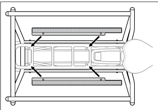
1. Align MadPad Plate to the top GSD rack mounting holes.
