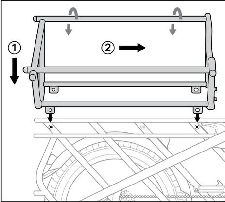
1. Insert the Clubhouse Frame at an angle to GSD rack. Rotate and slide into position.
