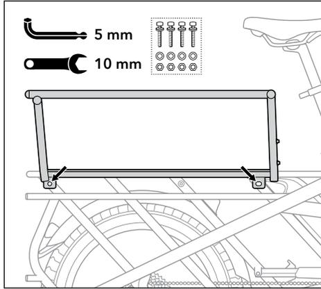
2. Align Clubhouse Frame to the side GSD rack mounting holes, insert M6 x 35 mm Bolts and tighten Bolts to a torque of 9 Nm - 10 Nm.
