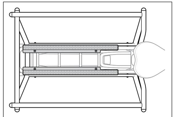
3. Tighten Bolts to a torque of 5 Nm - 6 Nm.
