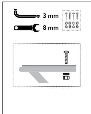
2. Insert M5 x 15 mm Bolts and partially tighten.
