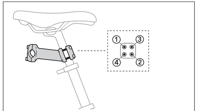
4. Place Faceplate onto Stem and tighten all bolts in cross pattern to a torque of 9-10 Nm.
