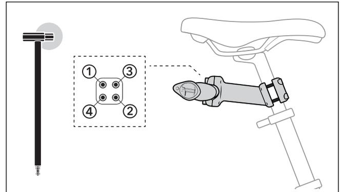
5. Tighten bolts in cross pattern to a torque of 9-10 Nm.
