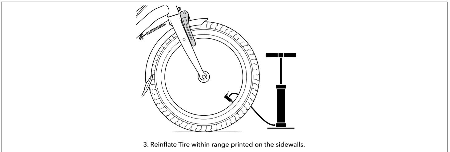
3. Reinflate Tire within range printed on the sidewalls.
