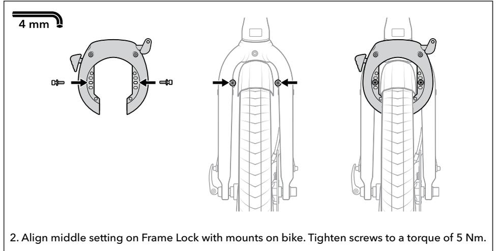
2. Align middle setting on Frame Lock with mounts on bike. Tighten screws to a torque of 5 Nm.
